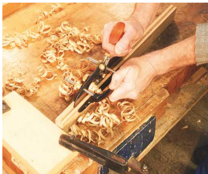
▲ Pic.12 Ploughing a groove with a speciality plane
